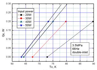
Figure 6. Cooling performance of dia.6 mm coaxial PTC with SS 400 mesh
