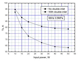
Figure 5. Change of refrigeration temperature with input power
