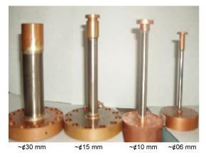
Figure 1. Photo of four coaxial PTCs with different regenerator diameters
