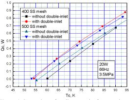
Figure 4. Comparison of cooling capacity for several cases
