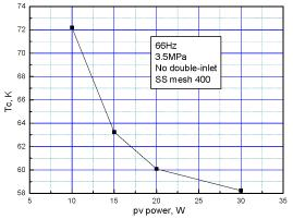
Figure 2. Change of lowest Tc with input pv power
