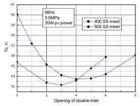
Figure 3. Effect of double-inlet on lowest temperature for two cases
