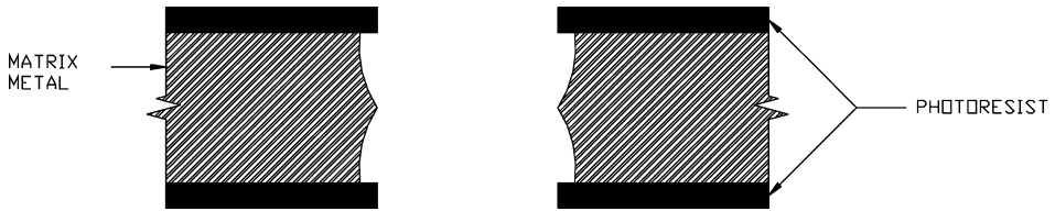
Figure 1. Schematic of channel section shape after chemical etching.
