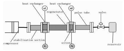
Figure 1. Experiment apparatus for testing the regenerators
