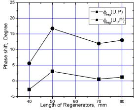
Figure 11. Phase shift of different regenerators
