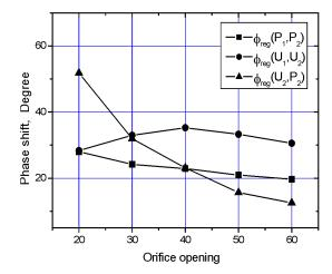
Figure 6. Phase shift depending on orifice opening
