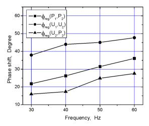
Figure 8. Phase shift depending on frequency
