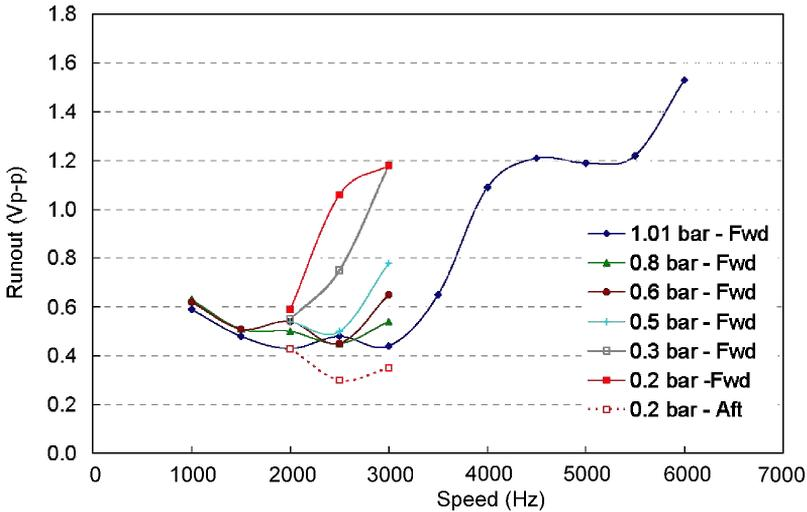
Figure 5. Shaft runout amplitudes during reduced pressure testing.
