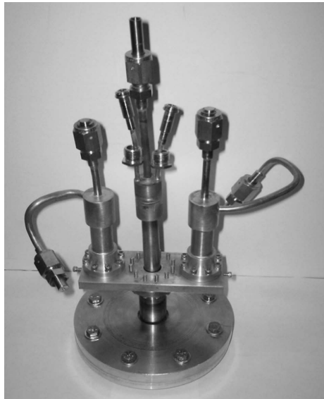
Figure 2. Pulse tube cold head, with Integrated Circulator installed, ready for testing
