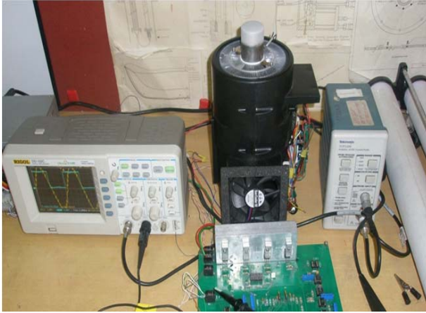
Figure 6. Photograph of the working TWINBIRD FPSC motor with analog PWM H-bridge inverter board. The ice formation can also be observed at the top most point of cold end. The setup was tested for continuous run of 8 hours. With a minimum temperature recorded during the test is -30^{\circ}\text{C} .
