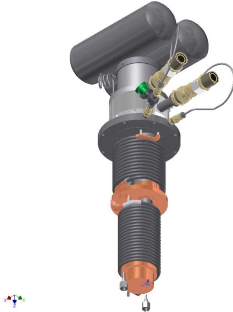
Figure 2. Design of the PT815 with cold helium circulation heat exchangers
