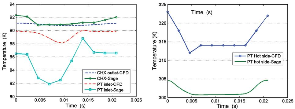
**Figure 4.** Temperatures (left) on the two ends of the cold heat exchanger (CHX) and (right) on the hot side of the pulse tube (PT)
