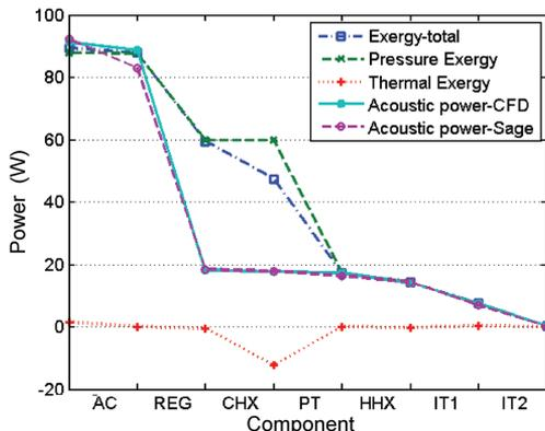
**Figure 5.** Exergy plots for aftercooler (AC), regenerator (REG), cold heat exchanger (CHX), pulse tube (PT), hot heat exchanger (HHX), inertia tube 1 & 2 (IT1 & IT2).
