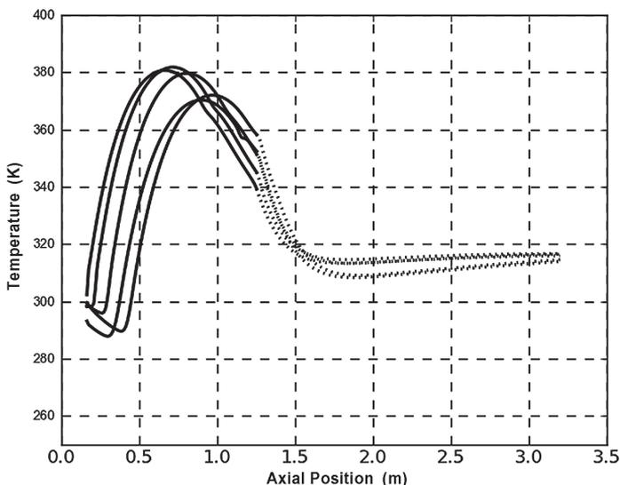
**Figure 6.** Temperature along the axis of the two inertia tubes (bold is IT1 and dotted is IT2) showing the temperature moving at different time steps.
