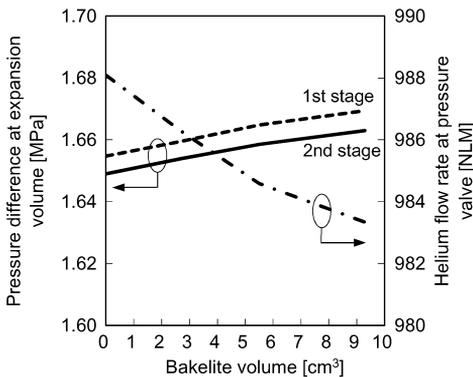
**Figure 7.** Calculated pressure difference at expansion volume and helium flow rate at pressure valve as a function of the bakelite volume for the Pb-rod.
