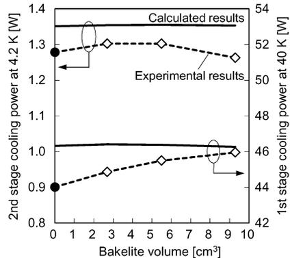
**Figure 8.** Comparison of the cooling power at 4.2 K and 40 K for calculated and experimental results of the Pb-rod.
