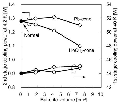
**Figure 6.** Comparison of the cooling power at 4.2 K and 40 K for the HoCu<sub>2</sub>-cone and the Pb-cone.
