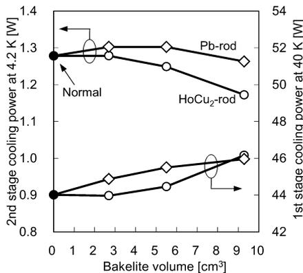
**Figure 5.** Comparison of the cooling power at 4.2 K and 40 K for the HoCu<sub>2</sub>-rod and the Pb-rod.
