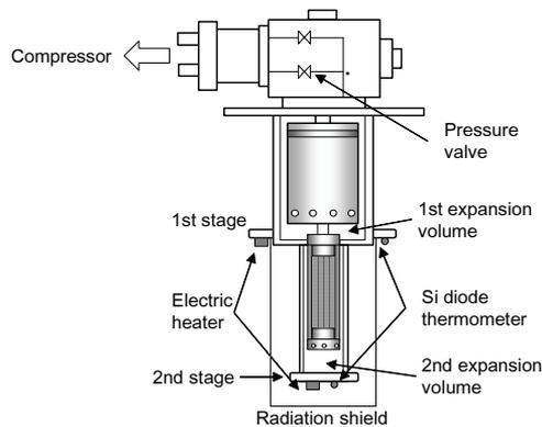
**Figure 1.** Schematic diagram of the two-stage G-M cryocooler.
