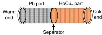
Figure 2. Two-layer configuration with Pb and HoCu<sub>2</sub> spheres: normal type.
