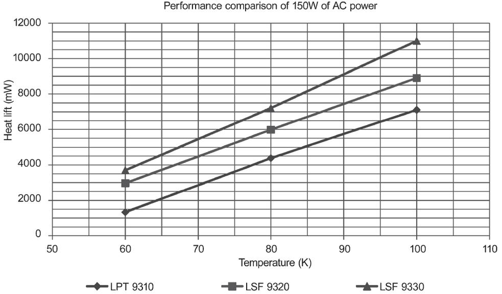
Figure 1. Load curves of LPT9310, LSF9320, LSF9330
