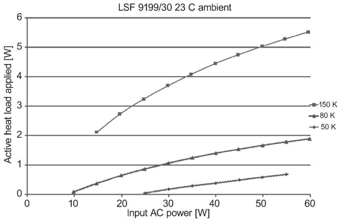
Figure 3. LSF9199/30 heat lift for various tip temperatures.
