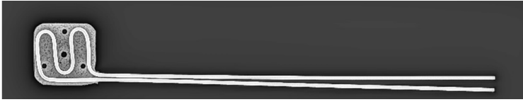
Figure 5. X-ray image of the cold trap before integration into the cryostat.
